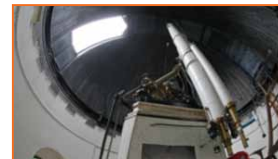
The great refractor (68cm lens and 10.5 focal length) at the observatory of the University of Vienna
