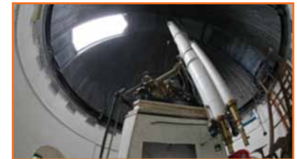
The great refractor (68cm lens and 10.5 focal length) at the observatory of the University of Vienna
