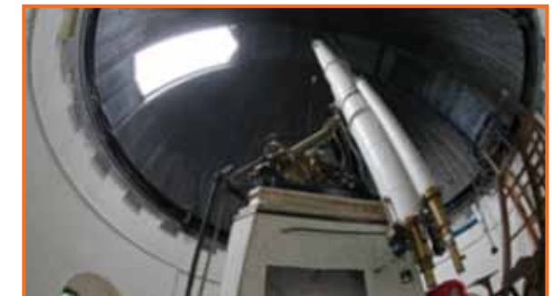
The great refractor (68cm lens and 10.5 focal length) at the observatory of the University of Vienna
